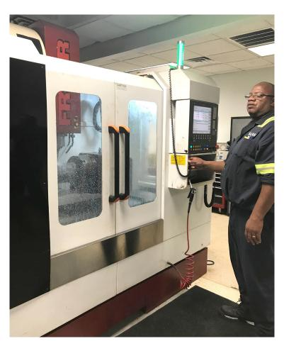
Using their Fryer MC-40 with a custom subplate with a 4th Axis set up, the QA shop cuts the DOGBONE, CHARPY specimens for testing. These were originally being done manually at an earlier facility using a knee mill and bandsaw.
